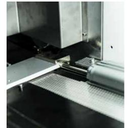
▲ The updated pin bar loading system has fewer moving mechanical parts, which minimises the risk of plate infeed problems and improves serviceability.
